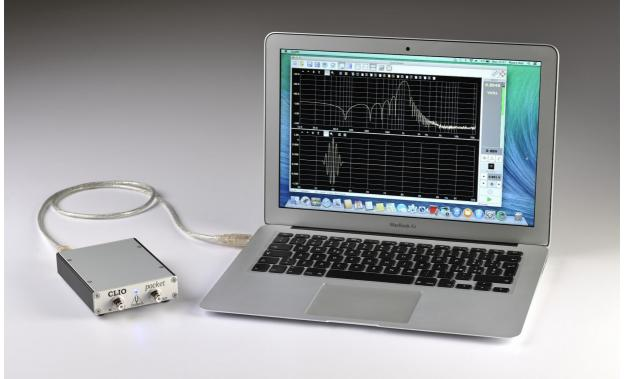
**CLIO Pocket** is Audiomatica's new Electro-Acoustical Multi-Platform Personal measurement system.
